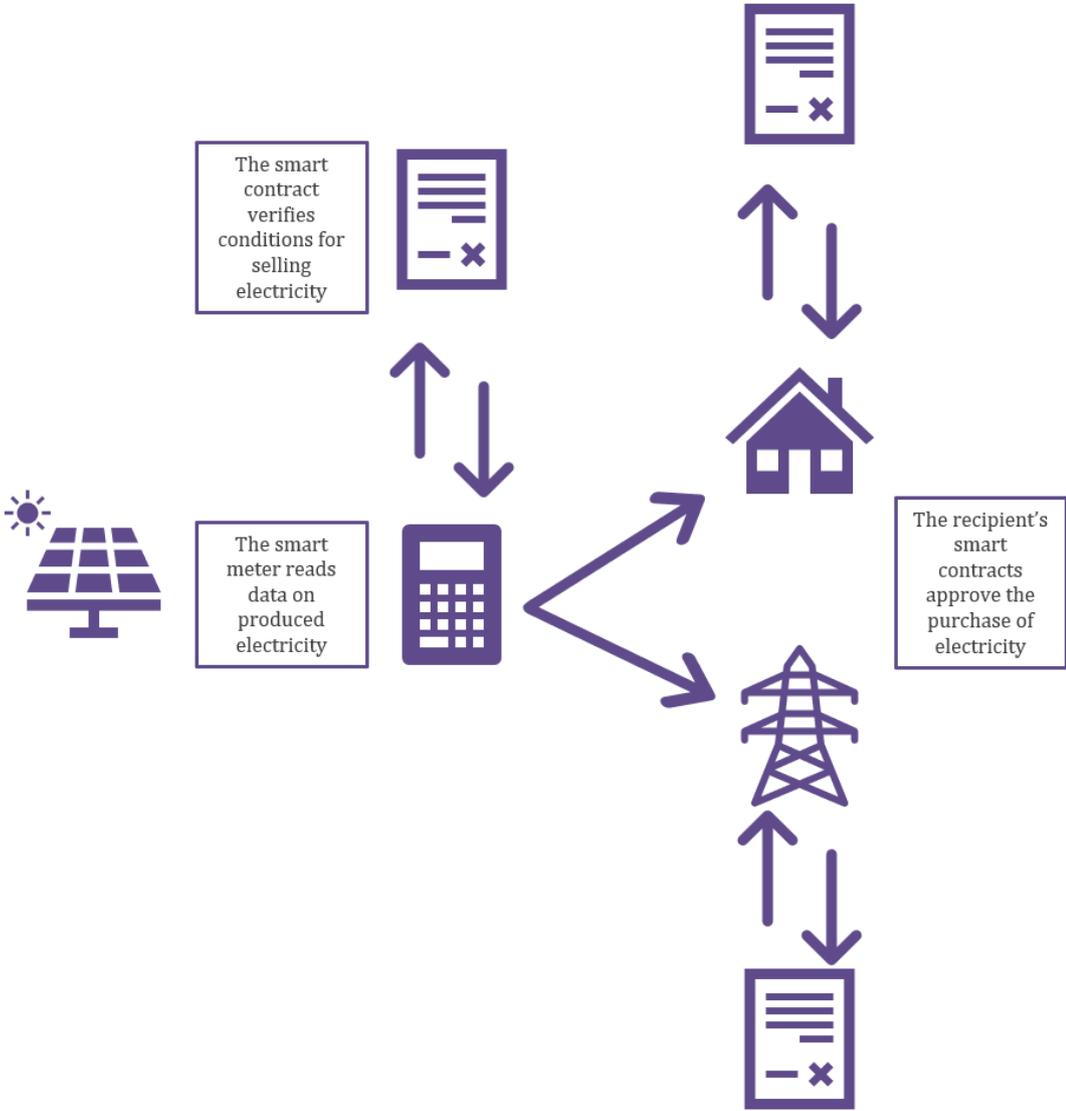
Figure 8: Example of a smart contract process for electricity trade [11]
