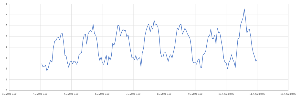
Figure 15. Sello's electricity consumption in MWh from 4.7.2021 to 10.7.2021. Source: Siemens
