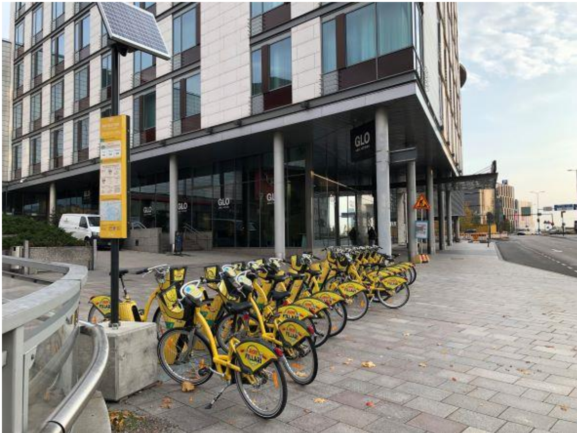
Figure 1. A city bike station, with bikes available for use, in front of the Sello shopping centre in Leppävaara (Leppävaarankatu). The PV panel that is integrated to the system feeds power to the digital locking mechanism of the bikes. Photo: author.
