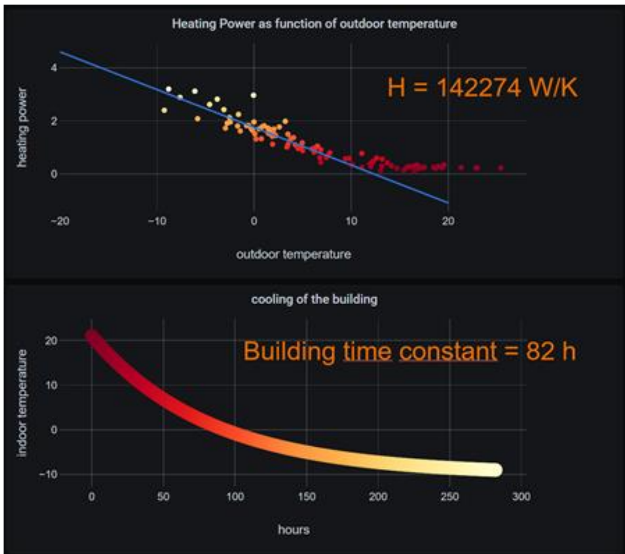
Figure 8. Time constant in Sello. H is the specific heat loss of the building spaces, and the time constant in Sello is 82 h. (figure from VTT)
